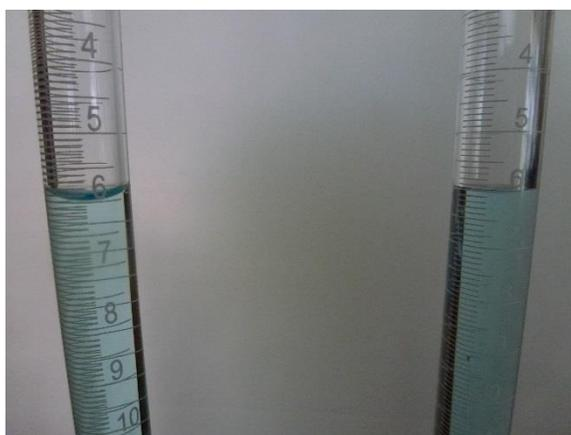
The scale divisions on a graduated cylinder are generally determined by its size. For example, the 50-mL graduated cylinder is divided into 1 mL increments. However, the scale of a 10-mL graduated cylinder is divided into 0.1 mL increments, and the scale of a 500-mL graduated cylinder is divided into 5 mL increments.
