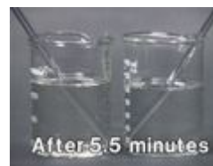
The other solution's reaction rate eventually increases as it forms manganese(II) ion, which subsequently autocatalyzes its own formation.
